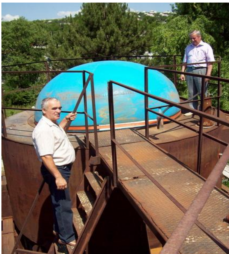
Bioreactor Anaerob Industrial-Experimental volum 34 \text{ m}^3
